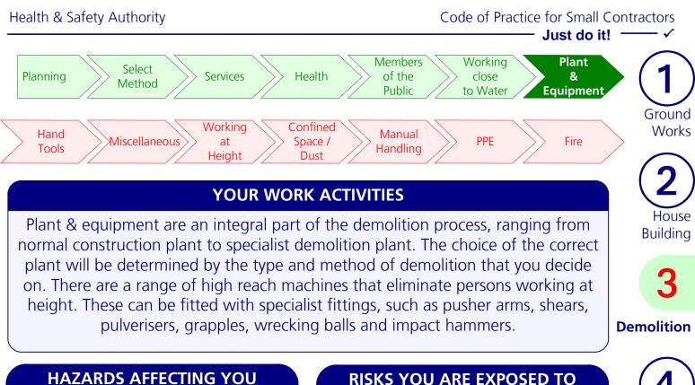
Plant may be exposed to overturning and destabilising loads during demolition. The use of specialist attachments will require competent drivers to use the plant and at a safe distance from material that can fall during demolition.
