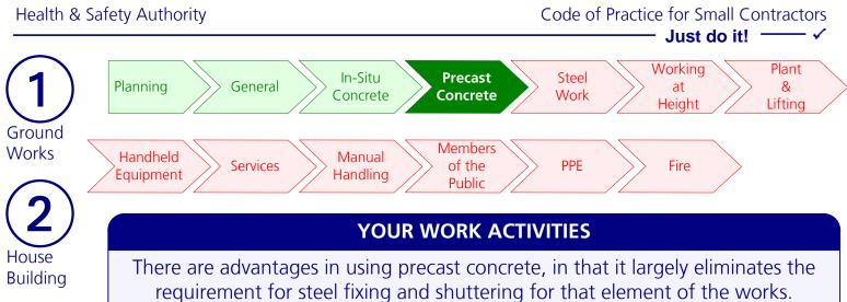
However one consideration is that the structure may be unstable, until all components are interconnected and acting together. Precast concrete will involve the delivery and lifting of large heavy units, which will have to be taken into account when planning the site layout and other work activities.
