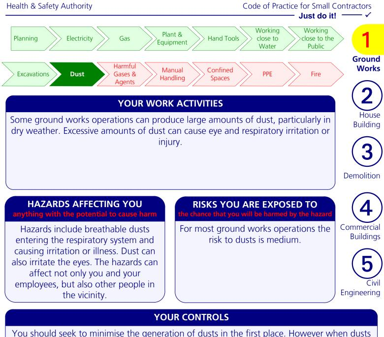
are generated by your work activities you should wet or damp down the area to prevent the dusts from becoming airborne. When working in confined spaces you should provide a fresh air supply to the work zone. A further control is to use a local exhaust system to remove the dust at source.
