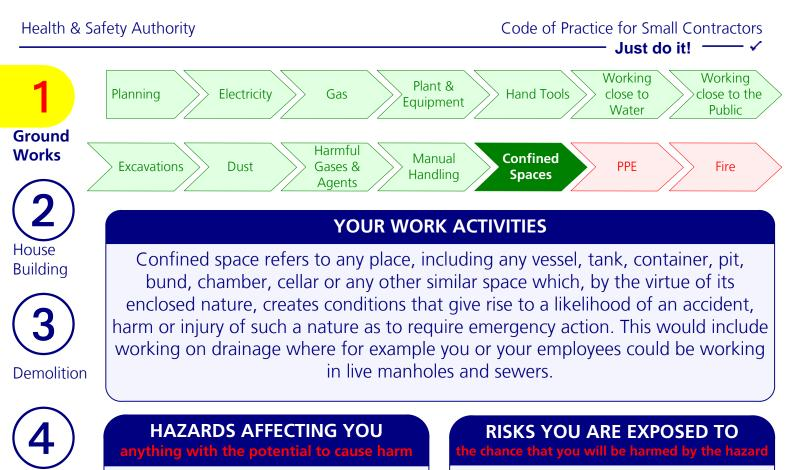
Any work in confined spaces exposes you or your employees to significant hazards, particularly where harmful gases or biological agents are present or can accumulate. The extent of the hazards can be compounded by the difficulty in providing assistance.
